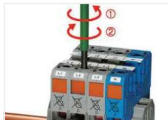
**Conductor termination (35 mm<sup>2</sup>) – step 3**
